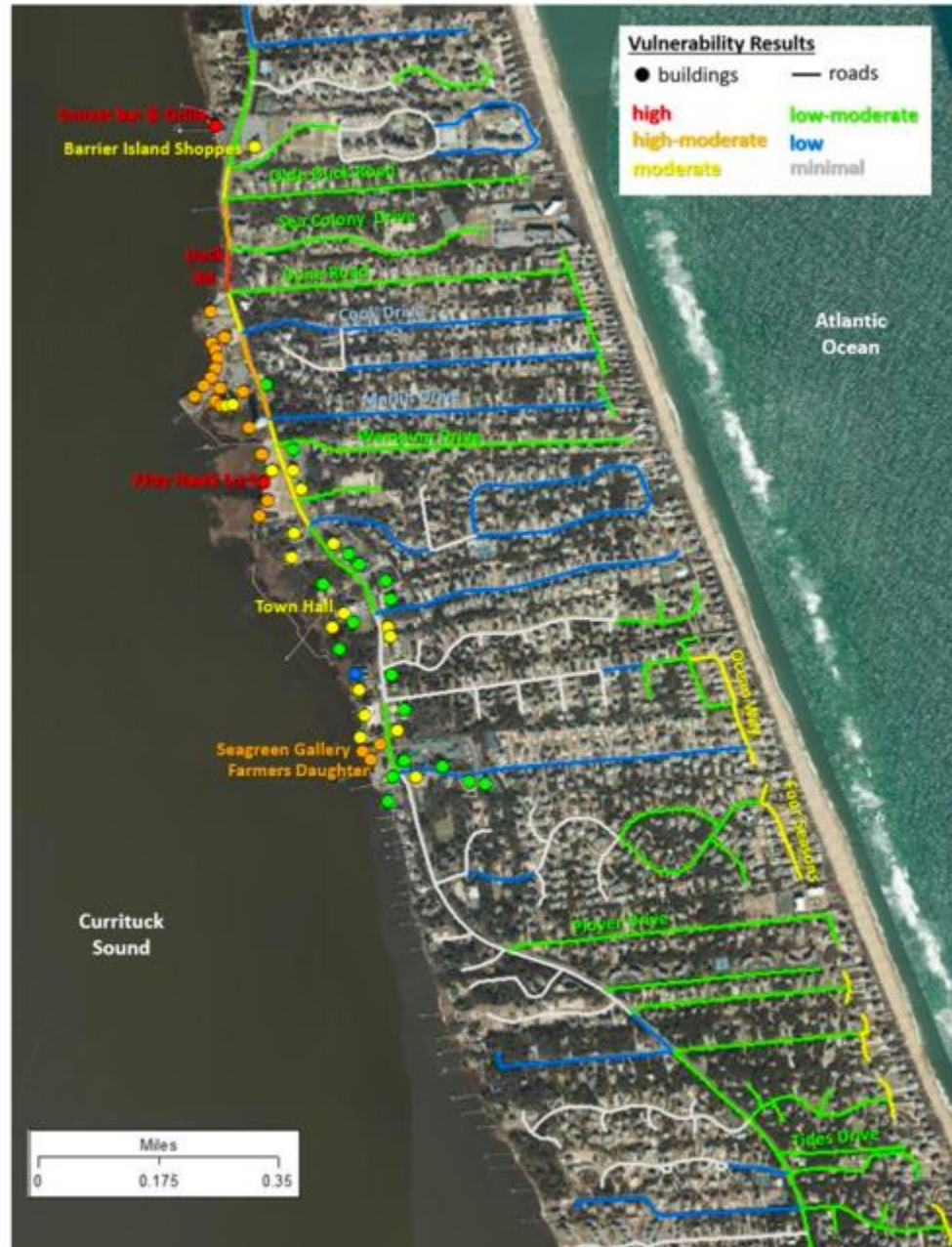
Figure 7. Coastal hazard vulnerability results for roads and select buildings in south Duck, near the town commercial center. Select assets are labeled.
